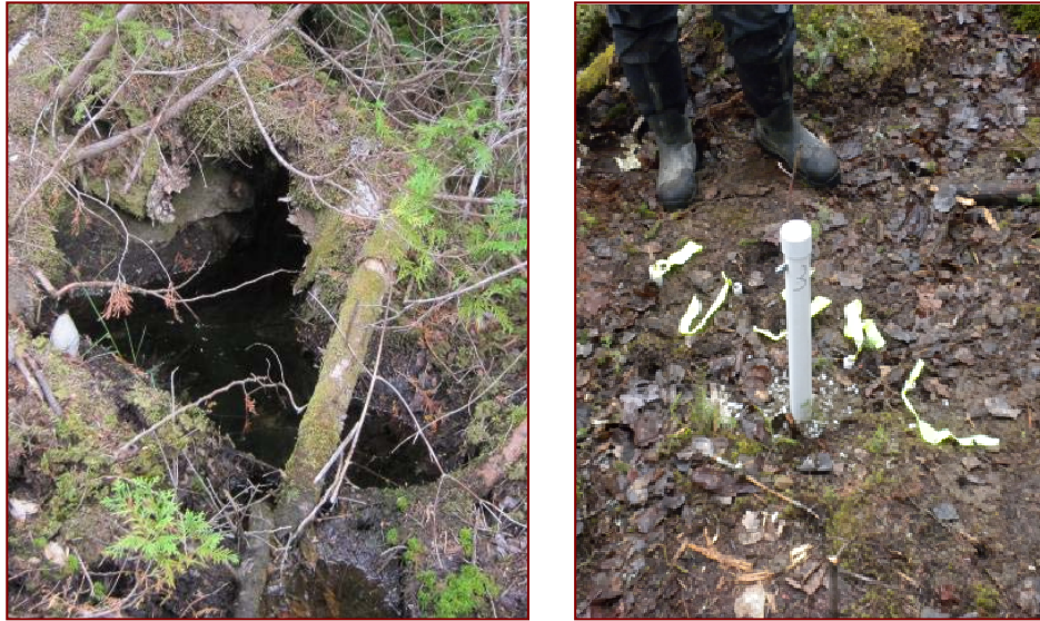
Figure 7. Sites with and without a separation between the folist layer and the soil surface. Left: Surfaces in which the moss and folist layer overlie the boulders and are separated from the soil surface, Burnt Jacket, Greenville, ME. Right: Monitoring well SB3, installed at a location that lacks a separation between the folist layer and the soil surface, Saddleback Mountain, Rangeley, ME.
