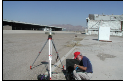
c. Established differential GPS base station used for precise trajectory information during LiDAR surveys.
